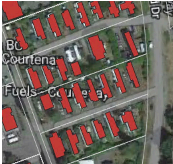
Figure 3-4: An example showing 27 building footprints are detected in a manufactured home park consisting of 4 land parcels.
